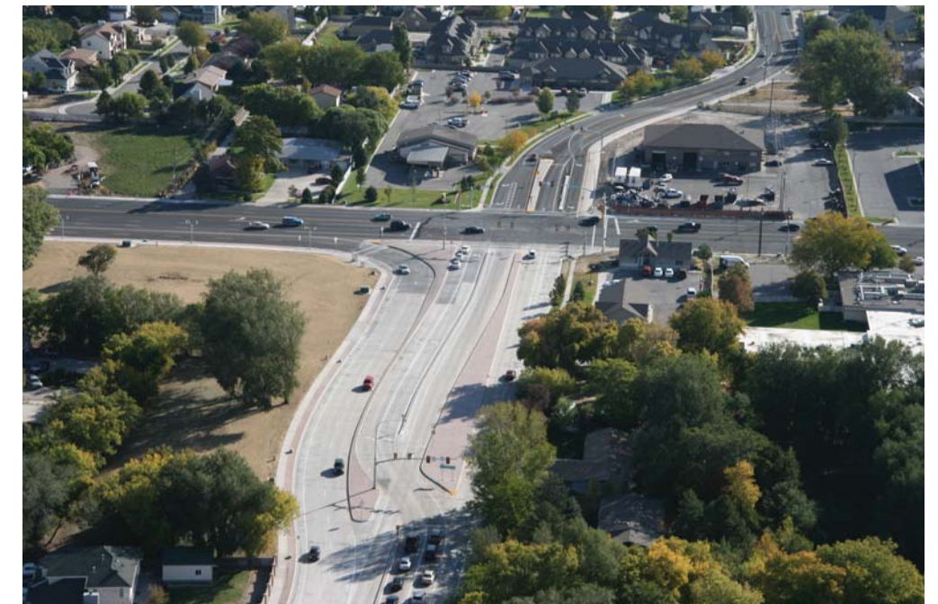
Figure 2-18 Continuous Flow Intersection
